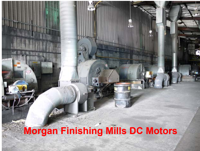
Morgan Stand 7 DC Motor and Gearbox
